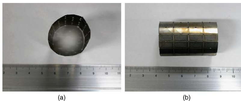
Fig. 5. Origami stent graft (a) projection and (b) side views before folding.
